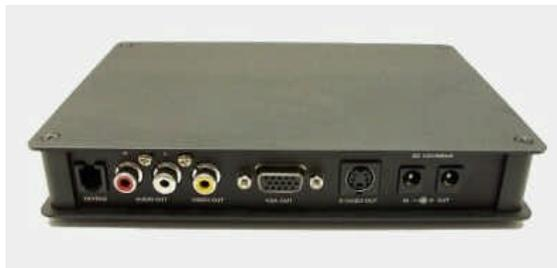
Plug in the RCA end of A/V cable to the jacks located at the rear of the DV-68 and then plug in the corresponding Yellow (Video), White (Audio L) and Red (Audio R) into the inputs on your monitor. Turn on power to the display and change the channel to the corresponding A/V input channel if necessary
